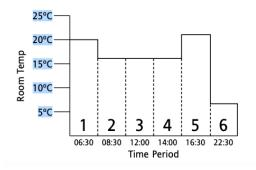
The standard programme on your thermostat is set for the temperature to rise to 20C at 6:30 in the morning, drop to 16C between 9am and 4:30pm, rise to 21C from 4:30pm to 10:30pm, then drop down overnight.
