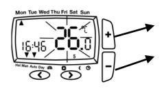
You can raise or lower these pre-set temperatures at any time simply by pressing the + or - buttons to the right of the temperature display. The temperature you select will flash for 5 seconds, then show the actual room temperature. Your new temperature will be maintained until the next period in the programme, when it will revert to the factory settings. You can then change the programmed temperature again in the same way.
