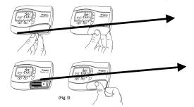
You can replace these by removing the battery cover with a coin.
