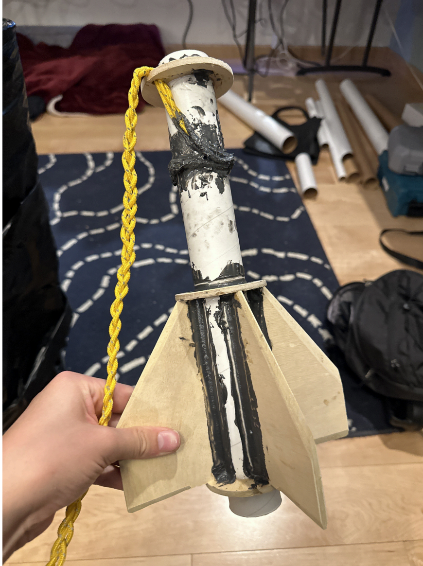
Completed motor mount assembly, with shock cord mounting and internal fillets visible.
