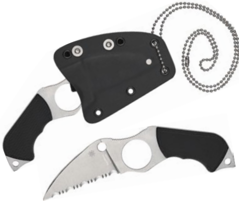
SCFB14S6 Swick 6 Fixed Blade. 5.88" (14.94cm) overall. 2.75" (6.99cm) satin finish LC 200 N tool steel serrated Wharncliffe blade. Black G10 handle. Full, extended tang. Lanyard hole. Finger ring. Thumb pull. Ball chain lanyard. Pistol grip style handle. Black Boltaron belt sheath. Boxed..... Retail $216.00
