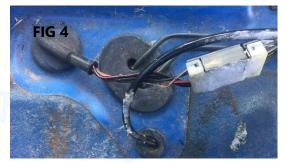
putting splice connectors and heat shrink on both ends of this snipped wire. See **FIG**
