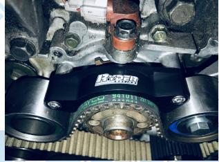
1) Remove the front Crank pully and timing belt covers as per OEM instructions. Remove the 2 x 10mm flange nuts from the top of the OEM timing belt guide, they can be discarded. Remove the Ryder Racing timing guide from the packaging and put in place of the original guide. Apply Lock Tight compound the threads of the cap head screws. Ensuring there is a minimum 1/16<sup>th</sup> gap between the
