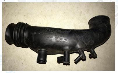
the inlet pipe to the inlet manifold, remove the EVAP control hose from the factory inlet pipe, remove the 3 x 10mm bolts from the rear of the inlet manifold. Disconnect the connector from the throttle body and place the connector aside, disconnect the bypass hose that connects to the factory inlet pipe, remove the spring clip from the crankcase
