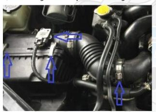
clamp on the inlet side of the factory turbo inlet hose. Discard this item unless it's already been replaced. Disconnect the plug from the AFM, unlock the two top tabs on the top of the airbox and place the unit aside (if the vehicle is equipped with an aftermarket CAI see the manufacturer for detailed removal of this section). If any connectors break please see our store for replacement items.
