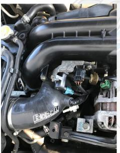
to the IC, fit the LHS bracket using the 3 x 12mm bolts, secure the worm drive hose clamp and secure the IC to the throttle body. Fit the bypass valve using the 2 x 12mm bolts and secure the last 12mm bolt on the righthand side.
