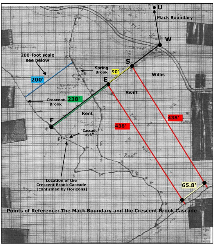
The 200-foot scale is faintly revealed between Crescent Brook and the Spring Brook. Thus, using that dimension, the scaled distance from E to F, the Kent back border, is approximately 238 feet. The surveyed distance by Horizons Eng. is 235'. Other distances by Horizons Engineering.
