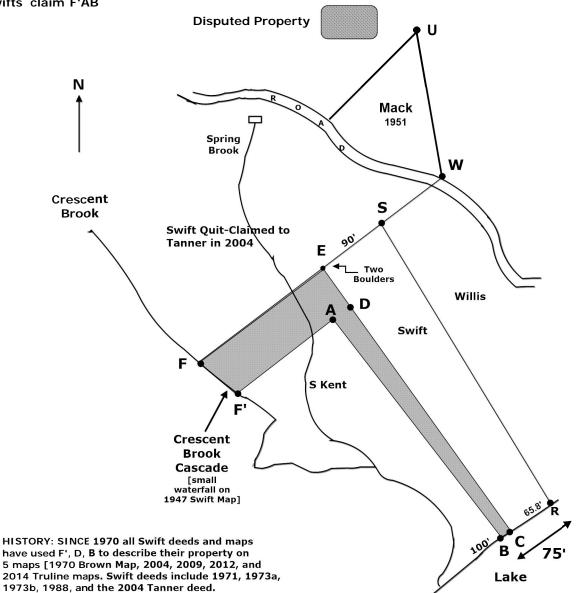
In 2012, Shane Clark, Swift's surveyor, discovered Pin A, and set Pin B 75' from Pin R [after Swifts retracted their claim of 81' which cut ~15' into the Kent beach frontage.] There has never been a Pin at location B.
