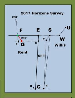
Conclusion: The "last mentioned boundary" coincides with the location of f<sub>b</sub> which is 231 feet from Stake E or no more than 4 feet from Crescent Brook. Given that the Defendants removed the incriminating paragraph from future land descriptions, and given that Stake G is missing, it is most probable that the boundary referred to was, in fact, the original Kent back boundary.
