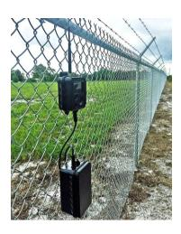
Built-in infrared triggers alert the OMNI GUARD cameras of activity. An image is quickly captured and sent to the guard station for your analysis.
