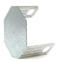
the ICFVL are embossed for additional stiffness and the hole allows for concrete to flow through and around the connector. The exposed flange on the face of the ICF provides a structural surface for mounting either a wood or steel ledger. <u>www.strongtie.com</u>
