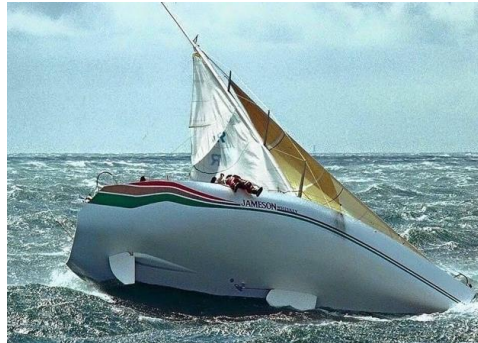
Fig.16 – A near-90° ‘knock-down’ of a similar yacht. Although such behaviour may seem ‘spectacular’, sailing yachts and their keels are expected to be designed and built to cater for such a scenario, and account for some movement during the event, that designers treat as “quasi-static”. This is not an instance of fatigue loading, which must be accounted for separately ( https://www.alamy.com/stock-photo-jameson-whisky-the-irish-entry-for-the-admirals-cup-broaches-in-breezy-31503836.html )
