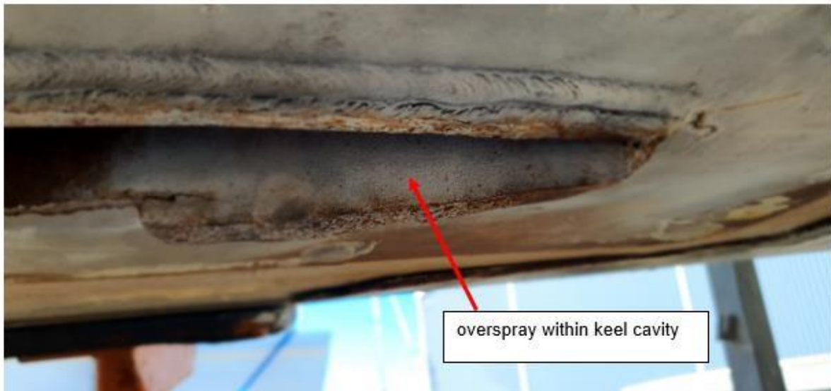
Fig.14 – White-coloured paint overspray within the keel cavity suggests that the keel had gaps in the welded connection of its root that let paint in. If present, gaps are also additional sites of crack initiation and promote further fatigue failure.
