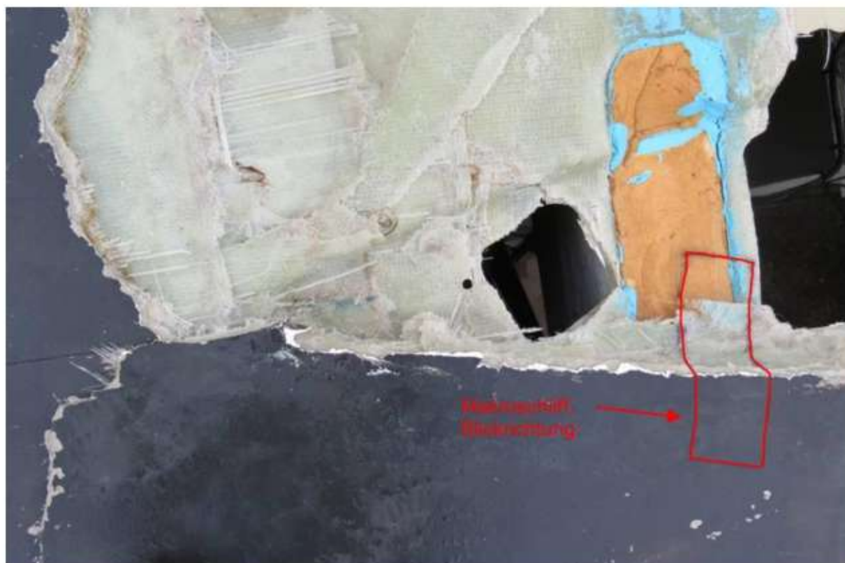
Photograph 5. The area where the material sample was collected from (source: GMA – 3664)
