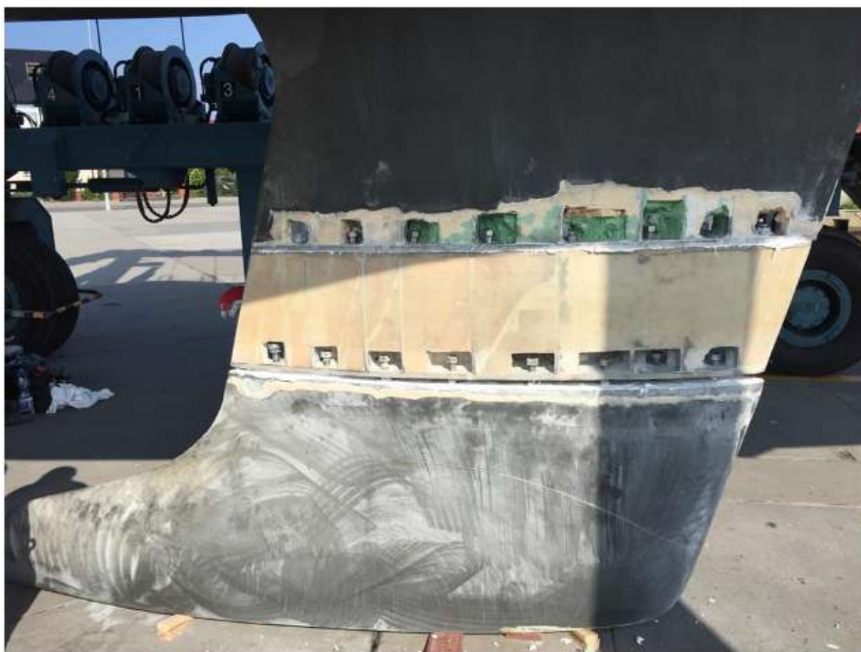
Photograph 15. Mounting of the bulb keel to the insert (source: yacht builder)
