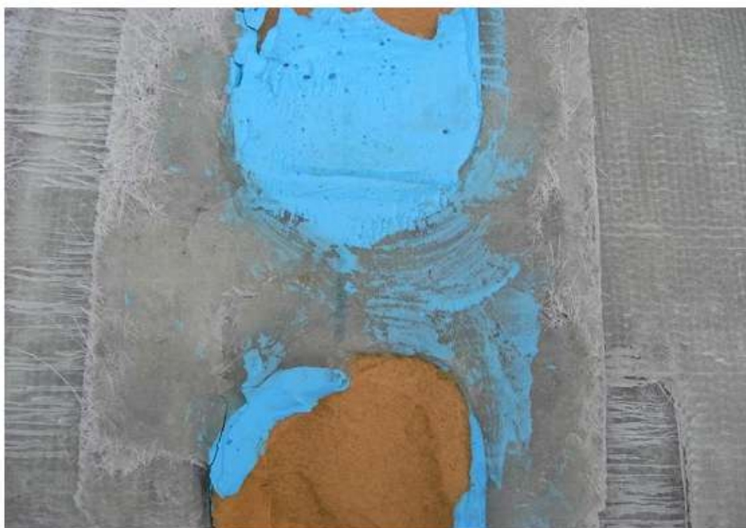
Photograph 10. Traces of glue outside of the bracing foam (source: Zucker & Partner GmbH report)
