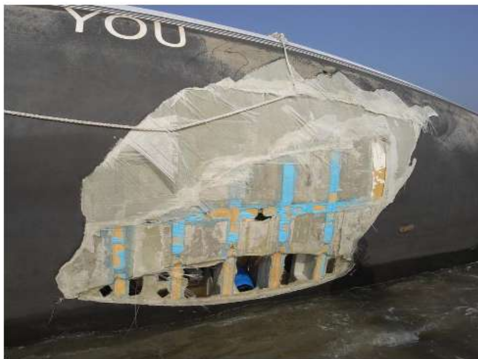
Photograph 11. Starboard view of the torn off recess and laminate layers (source: GMA-3664)
