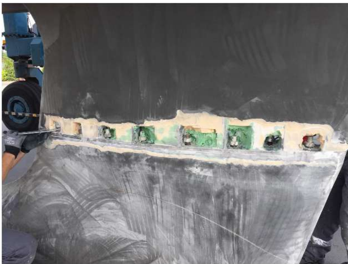
Photograph 13. Separation of the fin from the bulb keel (source: yacht builder)
