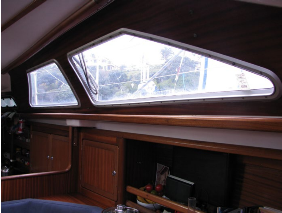
Photograph 5: Plywood storm coverings in position, but not secured over windows, on a Bavaria Oceans 47 sister ship
