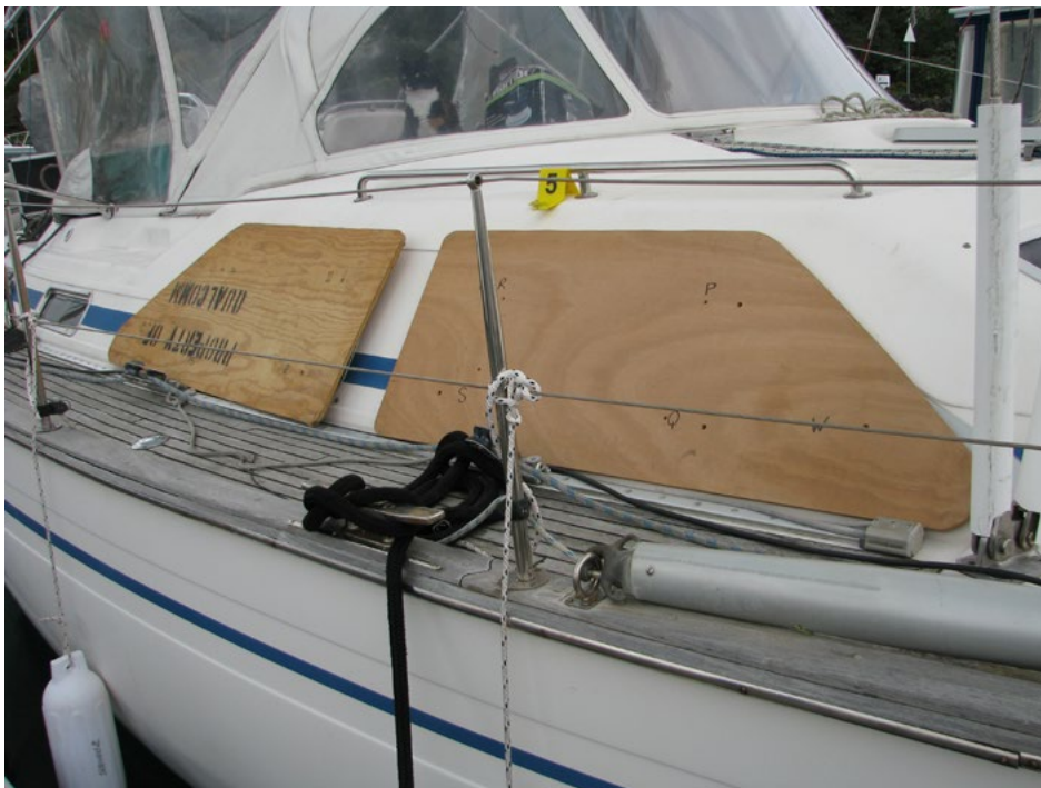
Photograph 5: Plywood storm coverings in position, but not secured over windows, on a Bavaria Oceans 47 sister ship
