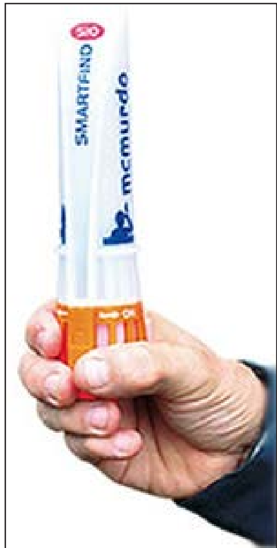
Figure 26: McMurdo S10 AIS beacon held in correct orientation
