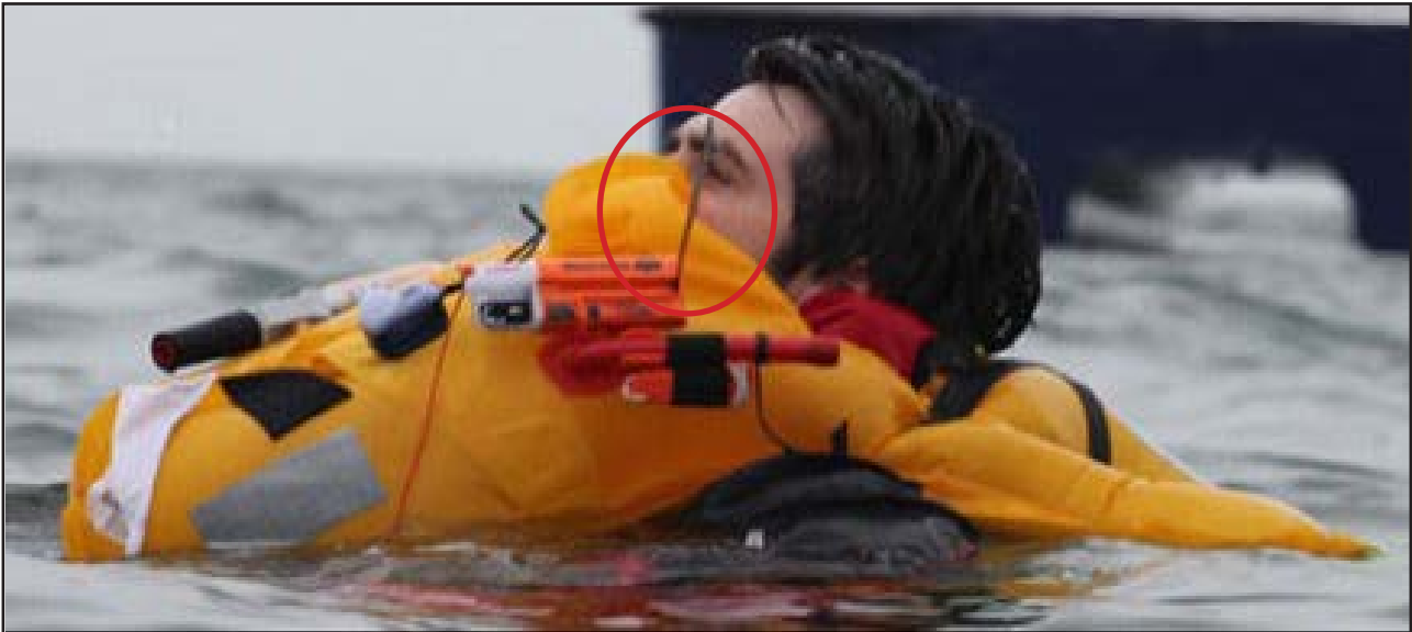
Figure 27: AIS beacon with antenna deployed on inflated lifejacket
