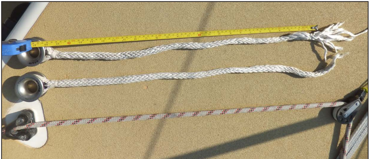
Figure 14: Failed preventer strop
