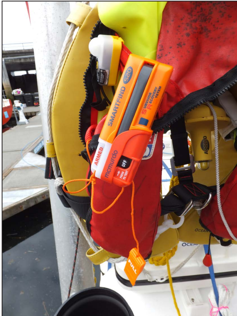
Figure 22: McMurdo S20 personal AIS beacon as rigged in Clipper lifejackets
