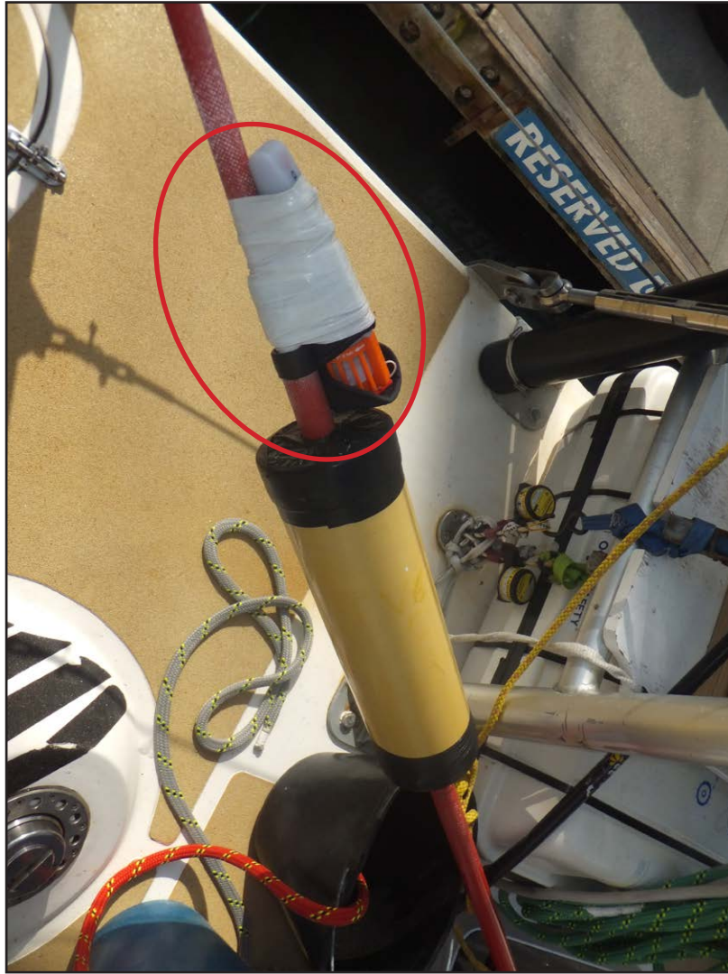
Figure 23: McMurdo S10 AIS beacon mounted on dan buoy
