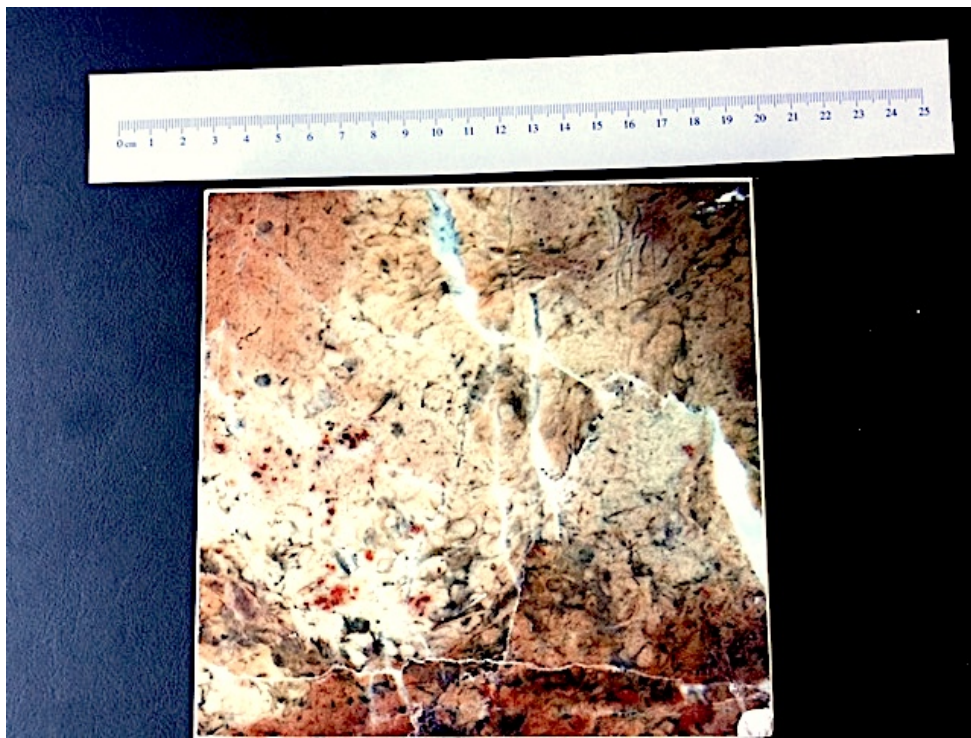
Figure 6: Example of marble pattern made by UV-printing the cement plate.
