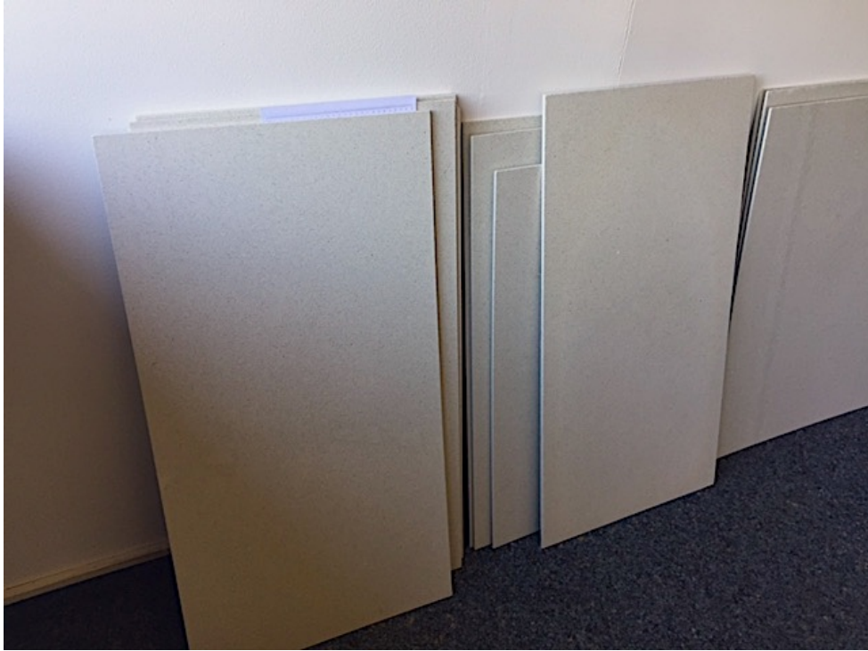
Figure 17: Example of full size extruded fiber cement panels.
