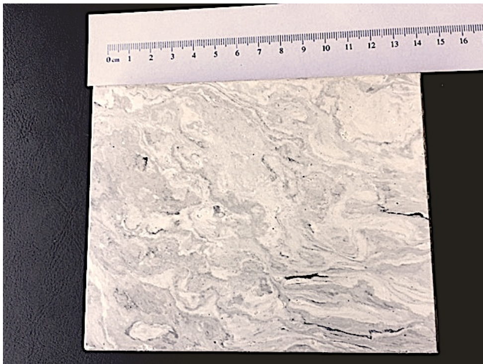
Figure 8: Example of marble-like pattern by mixing colors in the extruder.
