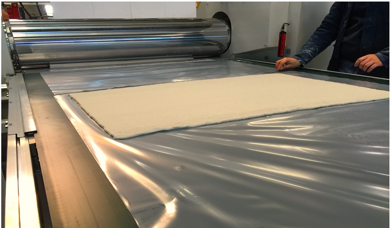
Figure 18: Cement panel produced on the pilot line.
