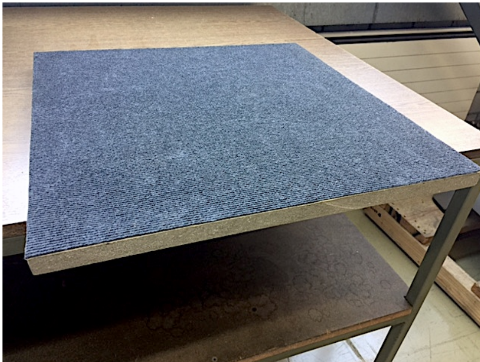
Figure 22: Example of extruded raised access flooring panel 60x60x2 cm.
