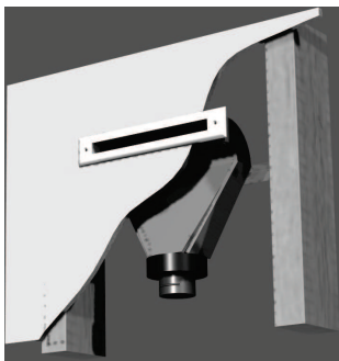
Figure 2. Typical Wall Installation, 90° Outlet
