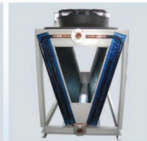
Dry Cooler (Air flow: 12,800 to 361,000 m 3 /h, capacity range: 27kw to 780kw) Cooling Medium: water + ethylene glycol, In/outlet fluid temp.: 44/39°C
