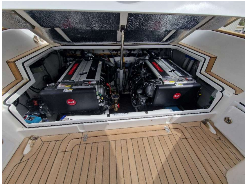
Engine room with the two main engines YANMAR
