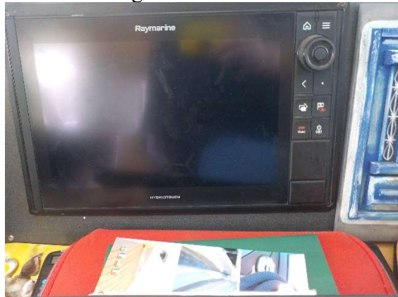
Below deck chartplotter / radar
