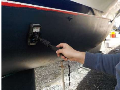
Moisture inspection with TRAMEX Skipper
