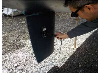
Moisture inspection with TRAMEX Skipper
