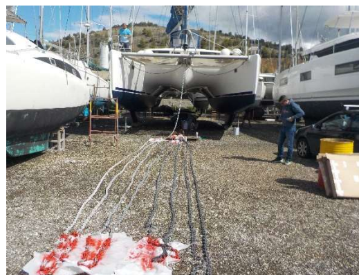
Anchor chain maintenance
