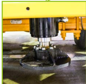
TOWER STABILIZATION WITH HYDRAULIC SUPPORTS
