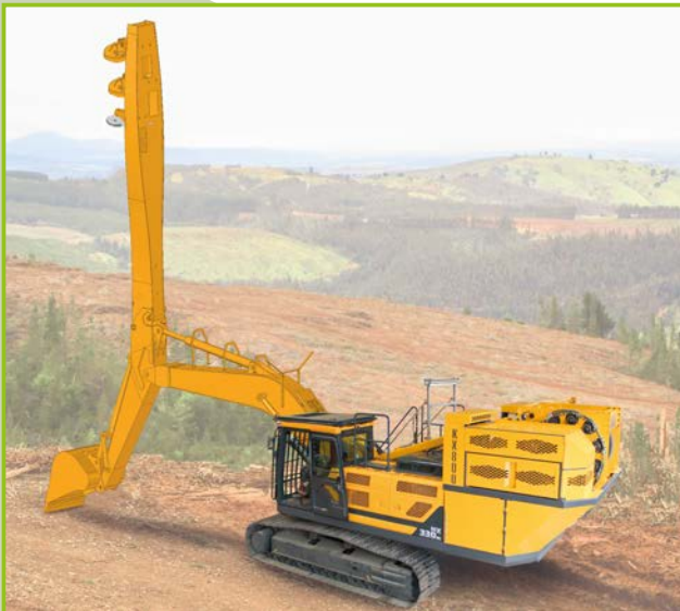
PULLEYS WITH BIG DIAMETERS
