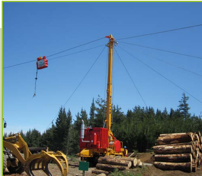
TOWER STABILIZATION WITH HYDRAULIC SUPPORTS
