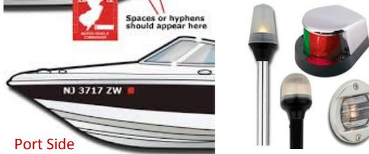
Navigation lights must be kept in serviceable condition and be displayed between sunset and sunrise and at times of restricted visibility.
