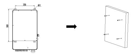
**Step 2**: Lift up the inverter and align the hole of the inverter with the expansion bolt, Fix the inverter on the wall.
