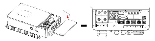
**Step 5**: Pass the corresponding conduit and fasten the joint.
