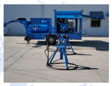
Mobile hardbanding units are portable welding units that can be used to apply hardbanding to drilling tubulars in the field. This can save time and money, as it eliminates the need to ship the tubulars back and forth to a service center.
