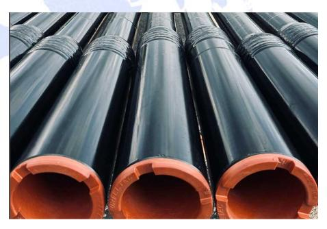
**Drill Pipe with New Thread Protectors**
