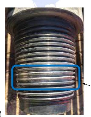
Minimizing the amount of weight applied to the connection during stabbing will reduce damage to the lead flanks of the tool joint threads.
