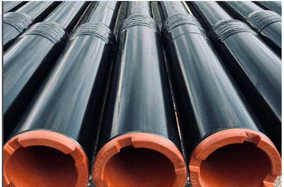
**Drill Pipe with New Thread Protectors**
