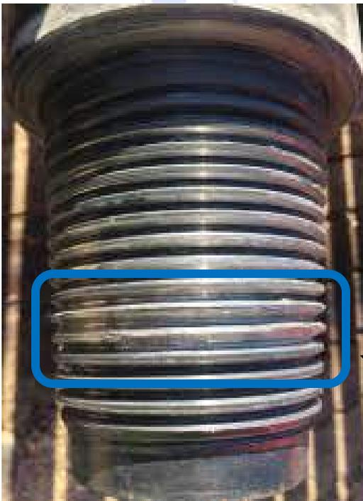
**Minimizing the amount of weight** applied to the connection during stabbing will reduce damage to the lead flanks of the tool joint threads.
