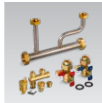
Combi-boiler primary manifold kit for NCB-H and NFC-H This package includes new stainless steel manifold, isolation valves with gaskets, PRV/air vent/LWCO adapter tree, air vent, threaded connection adapter with clip and LWCO plug. 30026576B
