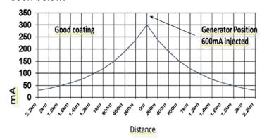
Where the coating is decaying or damaged, there is a significant increase in the rate of current loss. This is an increase in the Rate of Attenuation. In the figure below you can see a slight step change in the exponential curve of the AC signal.
