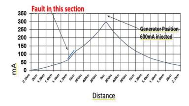
Shot locations can very along the survey chainage information is gathered via the on board GPS. The fault clearly seen below, in the logarithmic chart. The rate of current loss over any section of pipeline measured in millibels per meter (mB/m), is an absolute measure of the average quality of the coating over that section.
