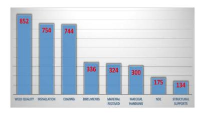
During a pre-backfill quality assurance interrogation led by a leading engineering company, the defects listed in the above chart were detected.
