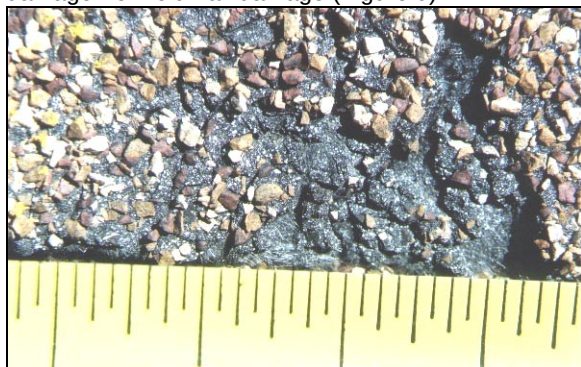
Figure 9. An example of 9-year-old hail damage to a glass-fiber mat asphalt shingle.
