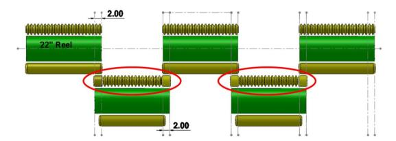
Multi-head mowers are designed with overlap positioning of the forward and rear reels causing double cutting of the turf that is typically visible as 2"-3" wide shadowing pathways or lines.
