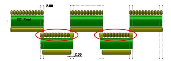
Multi-head mowers are designed with overlap positioning of the forward and rear reels causing double cutting of the turf that is typically visible as 2"-3" wide shadowing pathways or lines.
