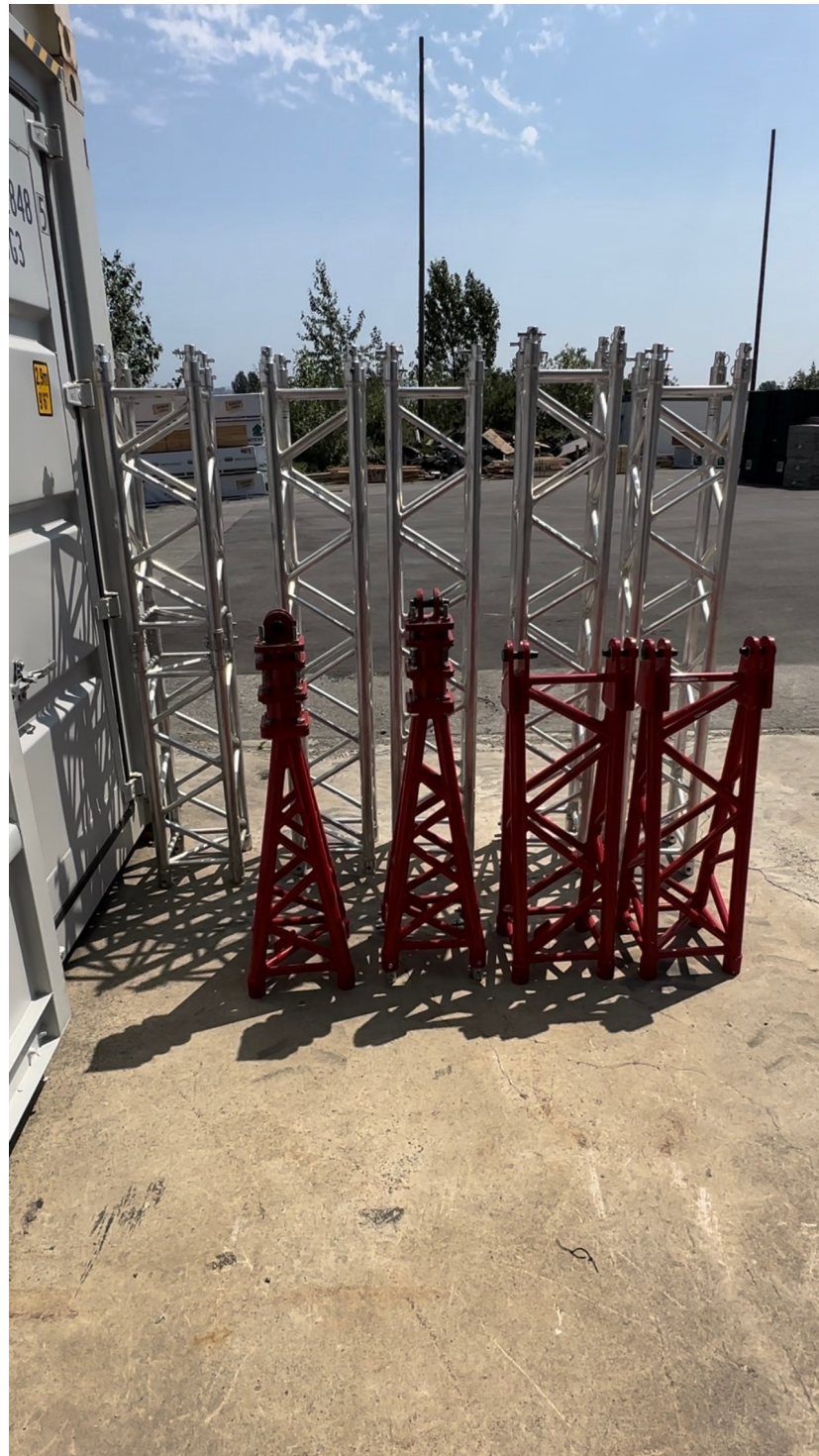
Components for 2 stiff-legs; container for scale
