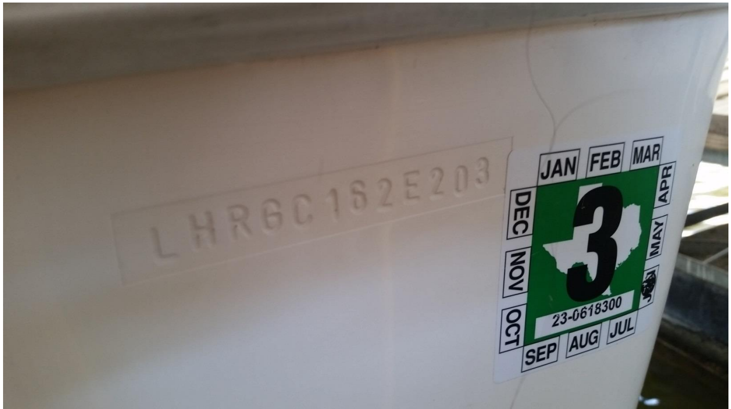
Hull Identification Number (Starboard Aft Corner under Rub Rail)
