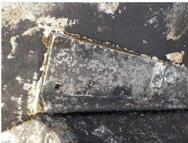
Missing Screws Port Trim Tab
