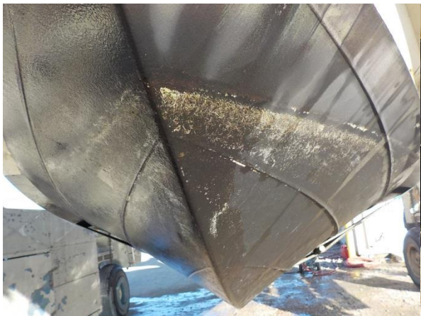
Bow Looking Aft Bottom Paint Flaking
