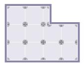
For pavers or tiles that are larger than 500x500mm, it is recommended that an extra paving support (with flat head) should be placed in the centre of the tile.
