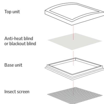
Mounting of blinds is done most conveniently during the rooflight installation process.
