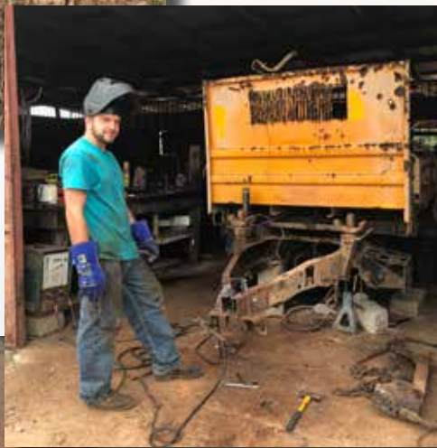
Lyndon changing the old dump truck into a dump trailer
