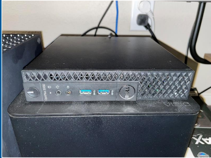
A home server made from a Dell OptiPlex
