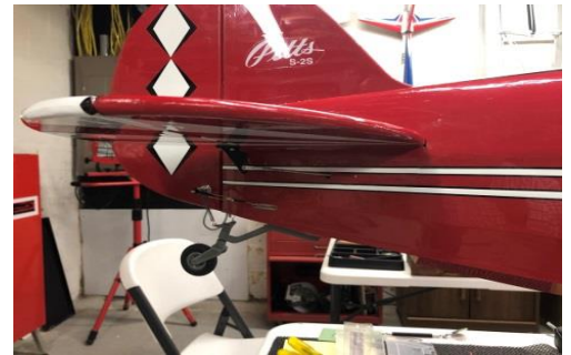
Lower wing aileron servos are concealed inside wing utilizing streamlined aluminum pushrods to operate the upper ailerons instead of separate servos. Elev. & Rudder servos concealed inside fuselage to enhance scale appearance.
