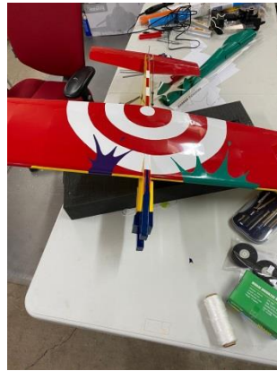
Ed's scratch-built U-Control Mamba started out as a 1/2a size model which he enlarged to a 40" wingspan with electric power. Covered with Monokote in the colorful paintball scheme. scheme.
