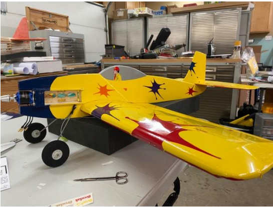
Ed's scratch-built U-Control Mamba started out as a 1/2a size model which he enlarged to a 40" wingspan with electric power. Covered with Monokote in the colorful paintball scheme. scheme.
