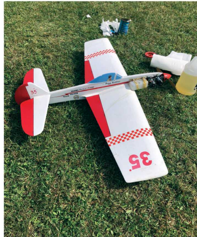
Dan Banjock's P-40Q CL Aerobatics model with a dual inline Fox .35 engine.
