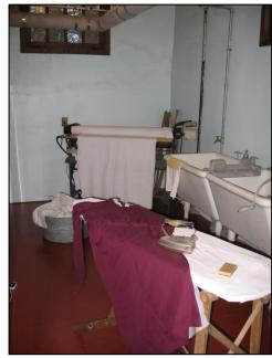
Dining Room located directly above it. The extra room was needed because laundry used to be a much more "hands-on" chore than it is today. The large machine in the corner under the window is called a "mangle." Operated by electricity, it used steam and hot rollers to iron the wrinkles out of flat linens such as tablecloths, sheets and pillowcases. It took a lot of skill to operate a mangle, a task that could be very dangerous for the untrained.
