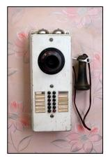
You can talk out of the building from any point or you can communicate to any station in the house or Garage without getting Central [Exchange]. The only disadvantage to this system, the servants can listen to any conversation if they want to and can also monopolize the use of the 'phone.
