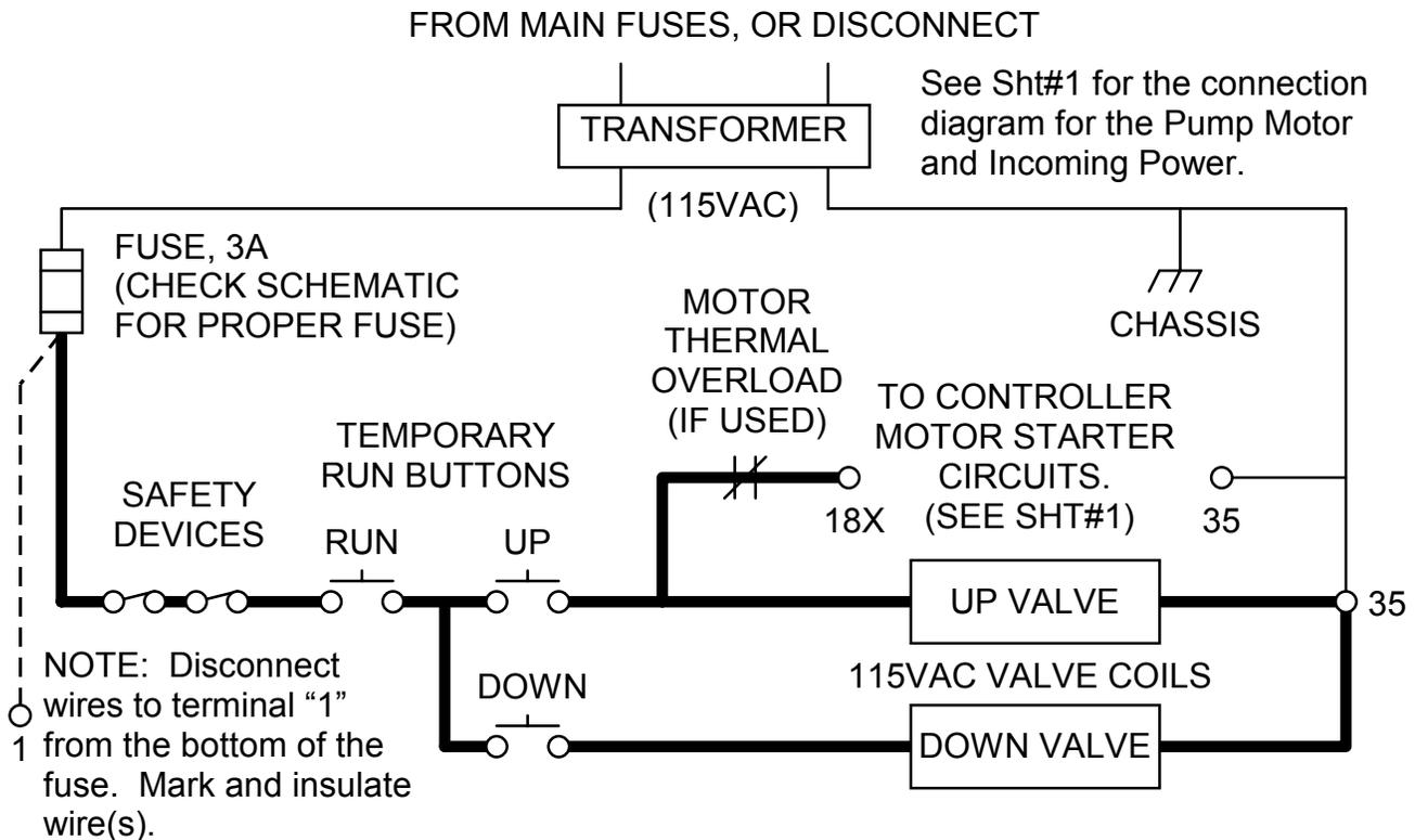
**WARNING: NO SAFETY DEVICES ARE SHOWN. CONNECT ANY SAFETY DEVICES AVAILABLE IN SERIES WITH THE RUN BUTTONS, AND USE EXTREME CAUTION WHEN OPERATING THE CAR.**
