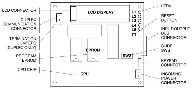
The Central Processing Unit (CPU) board contains the hardware that controls the inputs and outputs which control the elevator. This section describes the major components on the board, and the function of the connectors and LEDs. The operation of the Slide Switches labeled SW2 on the CPU are described below.
