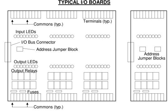
Input/Output boards are used to connect the CPU with the field devices. All inputs (unless otherwise stated) are 115VAC, and outputs (unless otherwise stated) are dry relay contacts.
