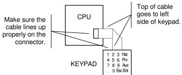
If the cable is plugged in incorrectly, then the keypad will not respond properly. Check the "Nxt" and "Prv" keys to see if the keypad cable is connected properly, since these keys should scroll through the menu items.
