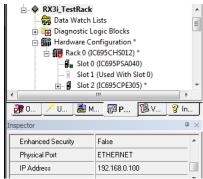
Through the Ethernet connection of an ETM001 in the same rack with a known IP address configuration.
