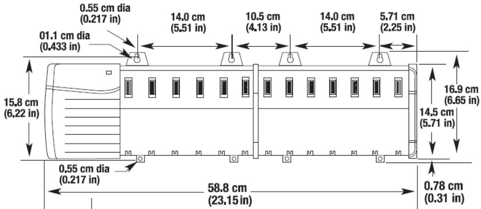
Figure 40 - Allen-Bradley ControlLogix #1756-A13 Chassis (with Power Supply)
