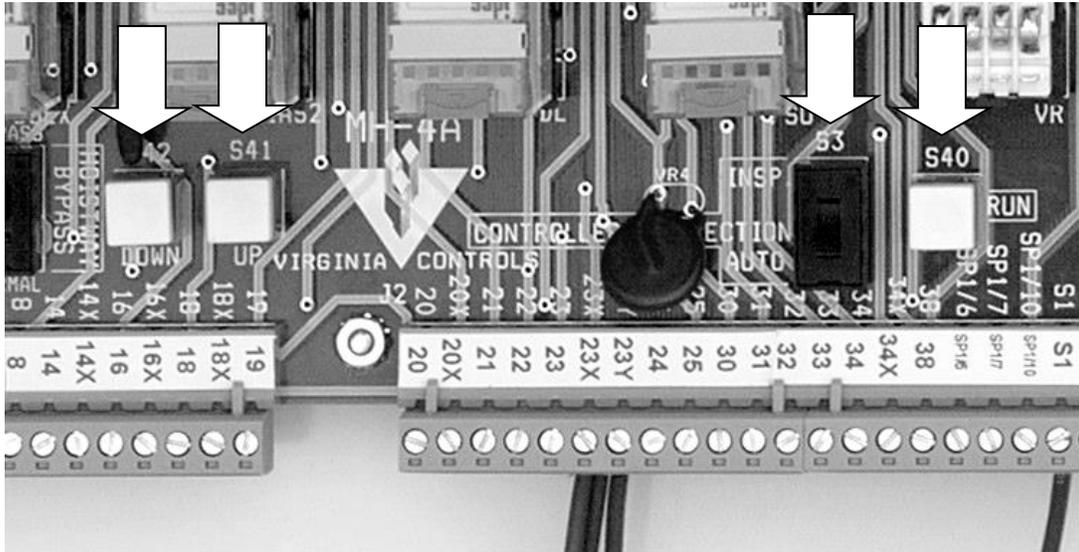
**Figure 51 - Inspection Switches**
