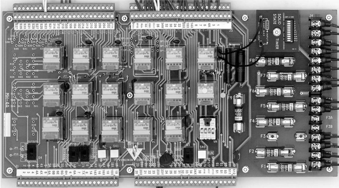
Figure 46 - MH4 Safety Interface Board
