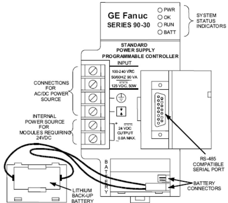
**Figure 7 - Standard AC/DC Input Power Supply - IC693PWR321**
