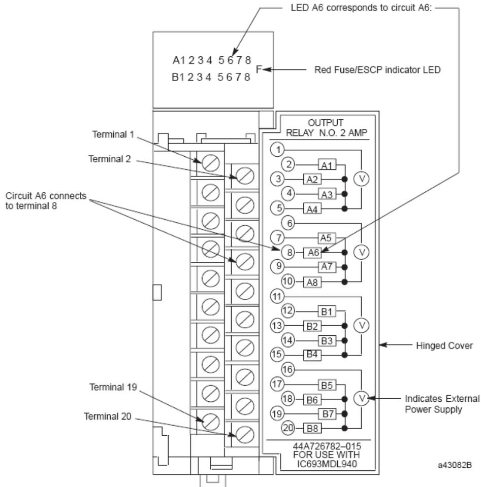
**Figure 8 - IC693MDL940 Standard Density Discrete Output Module**
