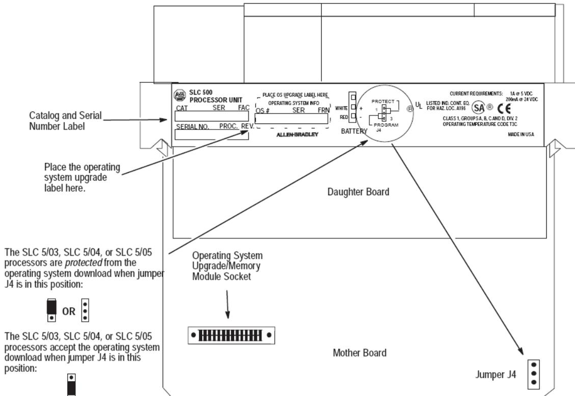
**Figure 15 - SLC 500 Processor Component Locations**
