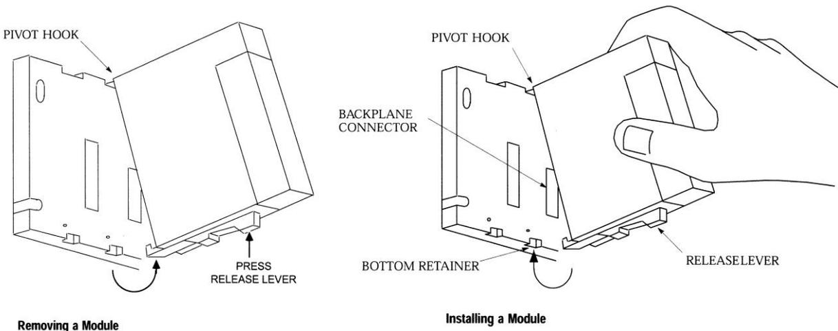
**NOTE: The Input and Output modules must be installed in the correct slots. The schematic indicates where each module should be located. Though Input modules may be changed with other Input modules of the same type, and Output modules changed with other Output modules of the same type, an Input module must never be put in a slot allocated for an Output module, and an Output module must never be put in a slot allocated for an Input module.**
