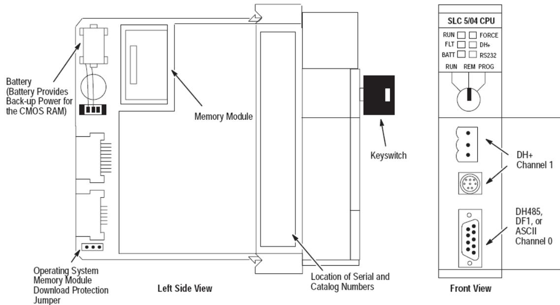
**Figure 13 - SLC 5/04 Processors (1747-L541, 1747-L542, or 1747-L543)**
