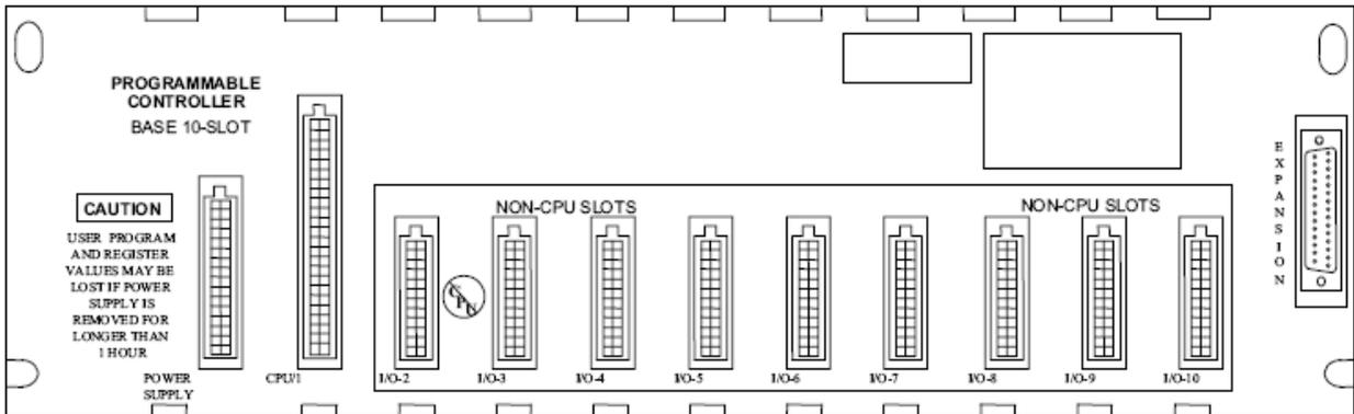
Figure 6 - IC693CHS391 10-Slot Modular CPU Baseplate
