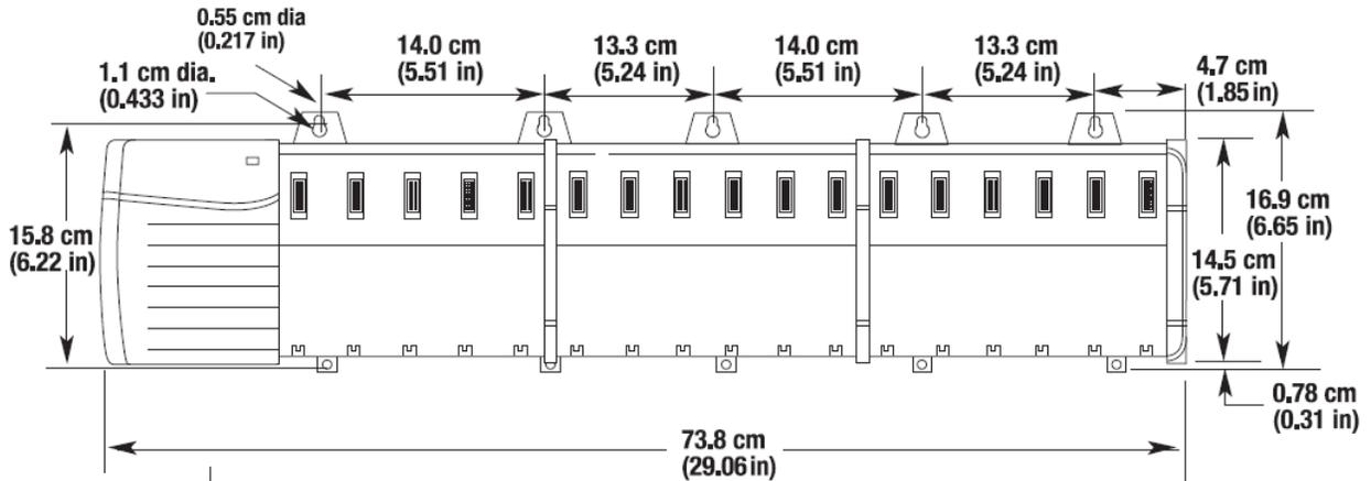
Figure 39 - Allen-Bradley ControlLogix #1756-A17 Chassis (with Power Supply)
