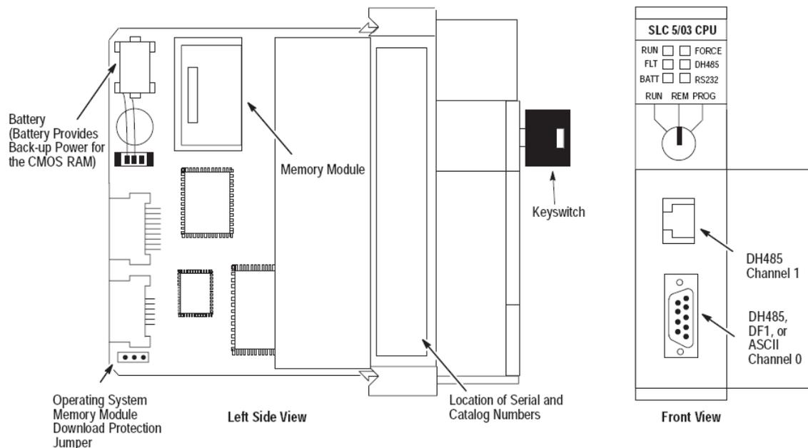
**Figure 12 - SLC 5/03 Processors (1747-L531 and 1747-L532)**
