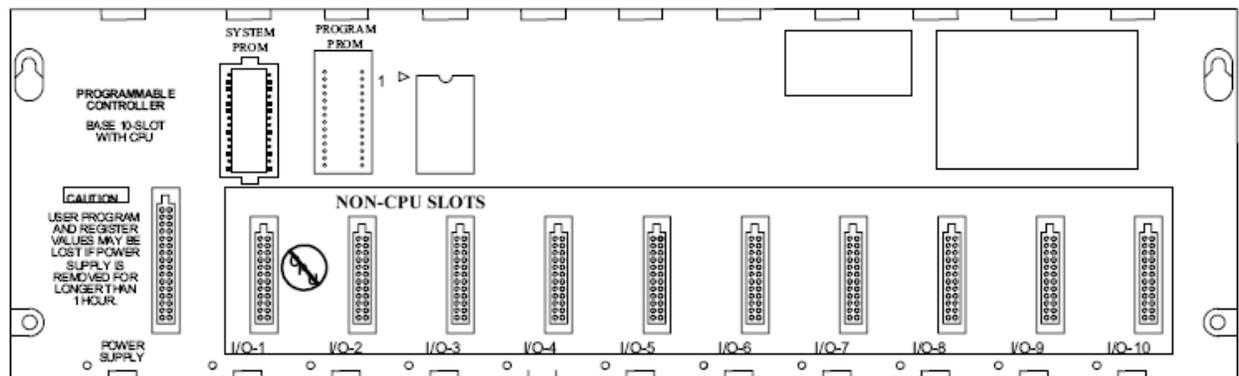
Figure 4 - Model IC693CPU323 (10-slot) Embedded CPU Baseplate
