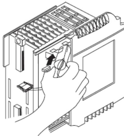
2. Insert the battery connector into the connector port. The connector is keyed to engage with the correct polarity.
