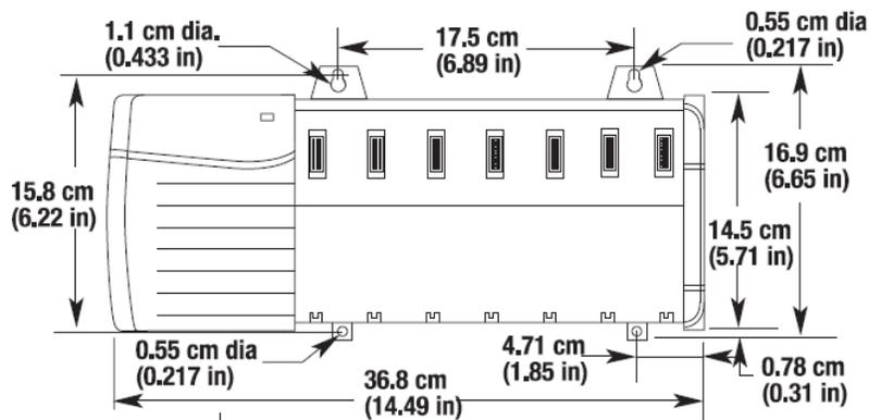
**Figure 37 - Allen-Bradley ControlLogix #1756-A7 Chassis (with Power Supply)**
