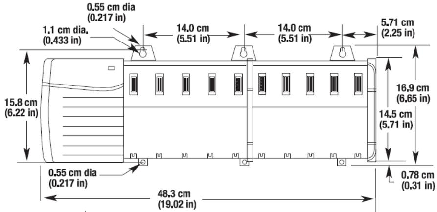
Figure 38 - Allen-Bradley ControlLogix #1756-A10 Chassis (with Power Supply)
