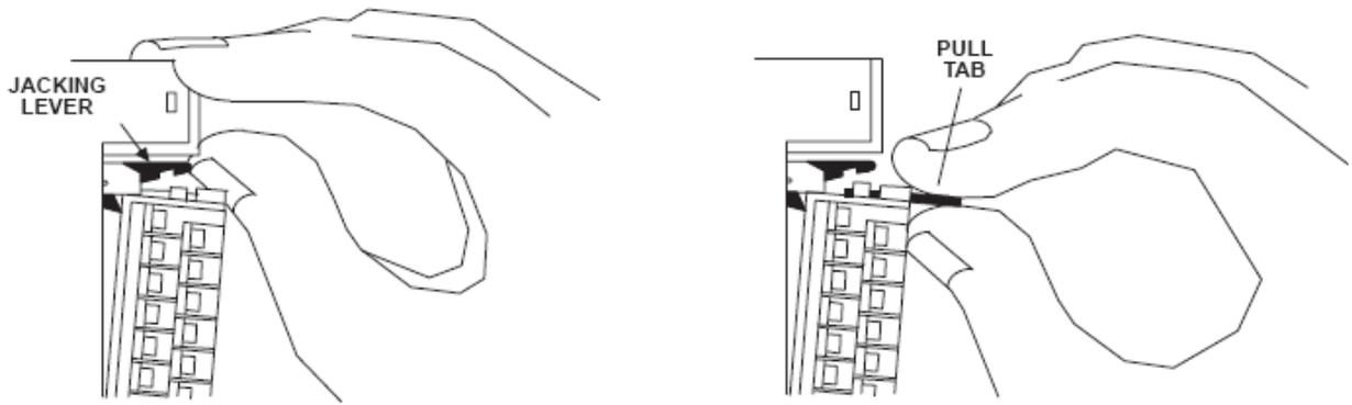
**Figure 9 - Removing 20-pin terminal assembly from module**
