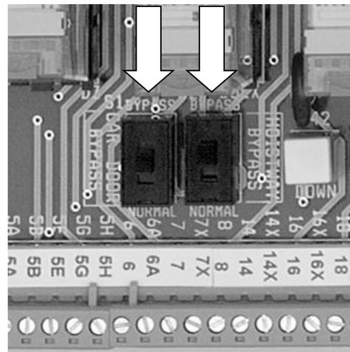
Figure 50 - Bypass Switches
