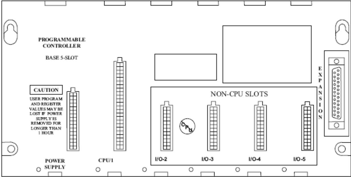
Figure 5 - IC693CHS397 5-Slot Modular CPU Baseplate
