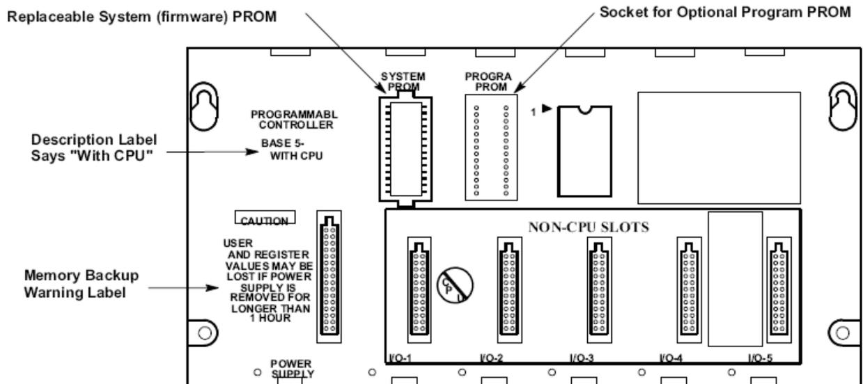
Figure 3 - Models 311 and 313 (5-Slot) Embedded CPU Baseplates
