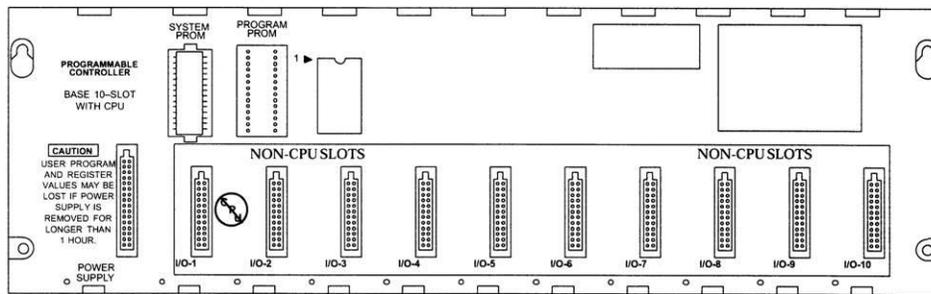
**Model IC693CPU323 (10-slot) Embedded CPU Baseplate**
