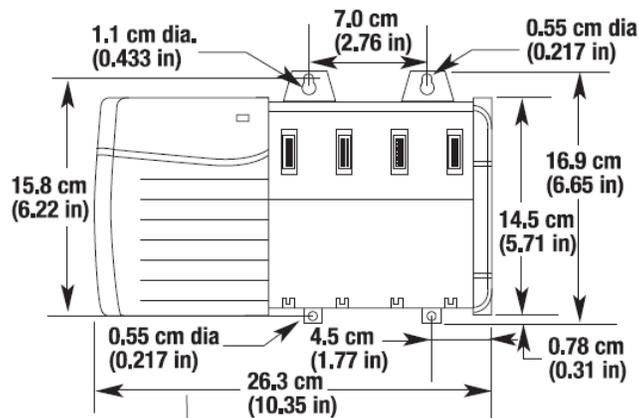
**Figure 36 - Allen-Bradley ControlLogix #1756-A4 Chassis (with Power Supply)**
