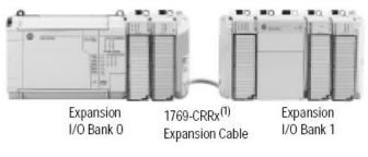
Figure 24 - Allen-Bradley MicroLogix 1500 Expansion (Horizontal Orientation)
