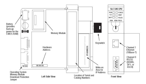
Figure 14 - SLC 5/05 Processors (1747-L551, 1747-L552, and 1747-L553)
