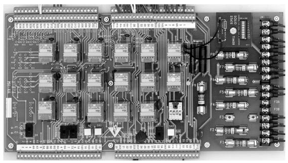
Figure 46 - MH4 Safety Interface Board
