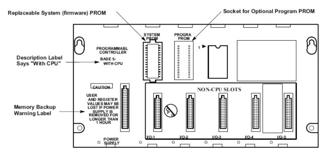
Figure 3 - Models 311 and 313 (5-Slot) Embedded CPU Baseplates
