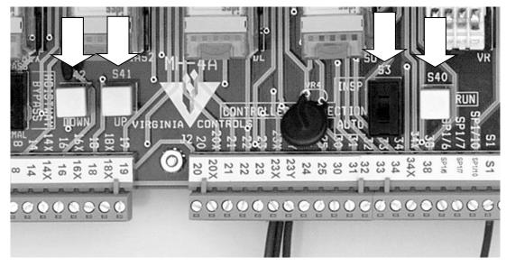
**Figure 51 - Inspection Switches**
