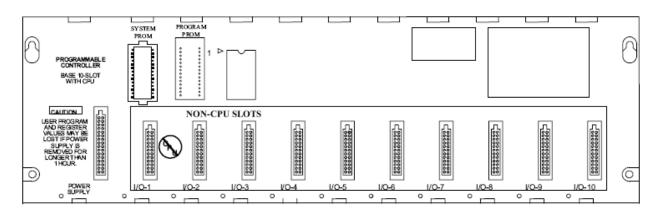
Figure 4 - Model IC693CPU323 (10-slot) Embedded CPU Baseplate
