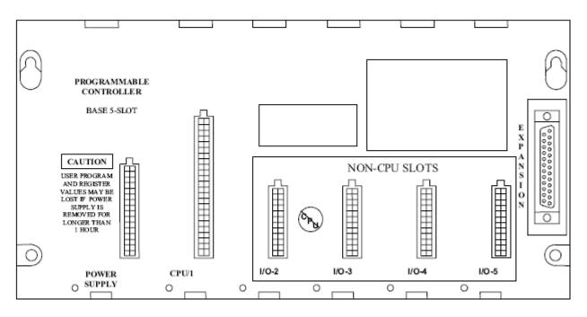
Figure 5 - IC693CHS397 5-Slot Modular CPU Baseplate
