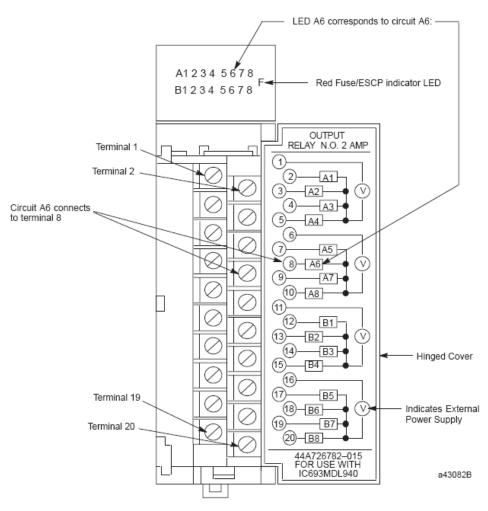
Figure 8 - IC693MDL940 Standard Density Discrete Output Module
