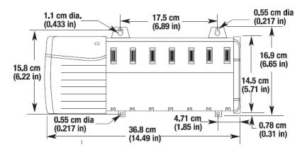
Figure 37 - Allen-Bradley ControlLogix #1756-A7 Chassis (with Power Supply)
