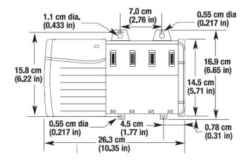
Figure 36 - Allen-Bradley ControlLogix #1756-A4 Chassis (with Power Supply)
