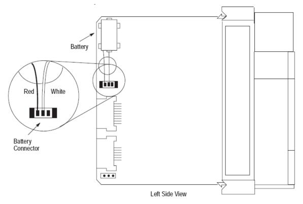
Figure 16 - SLC 500 Processor Battery Location
