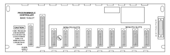
Figure 6 - IC693CHS391 10-Slot Modular CPU Baseplate
