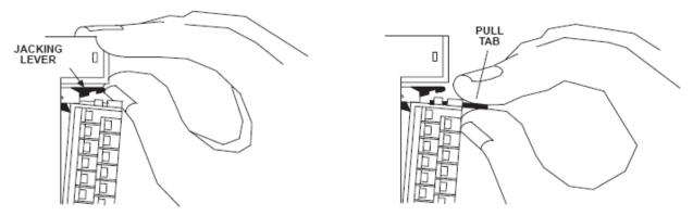
Figure 9 - Removing 20-pin terminal assembly from module
