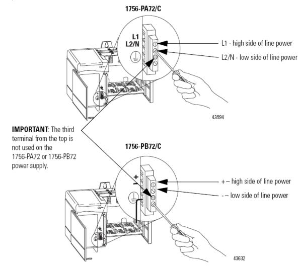
Figure 41 - Allen-Bradley ControlLogix Power Supply Wiring
