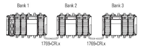
Figure 31 - Allen-Bradley CompactLogix (Horizontal Orientation)
