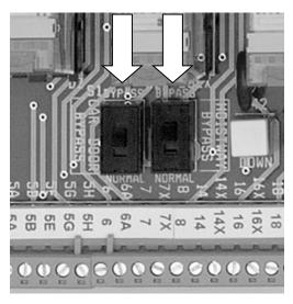
Figure 50 - Bypass Switches
