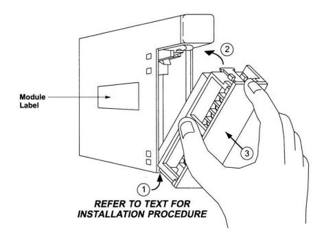
Figure 10 - Installing 20-pin terminal assembly on to module
