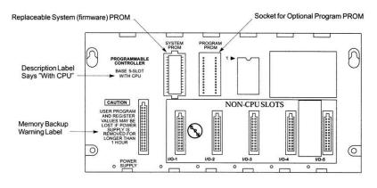
Models IC693CPU311 and IC693CPU313 (5-Slot) Embedded CPU Baseplates
