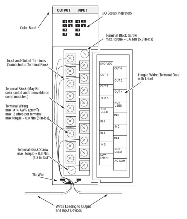
Figure 18 - Features of an Allen-Bradley SLC 500 I/O Module
