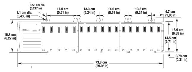
Figure 39 - Allen-Bradley ControlLogix #1756-A17 Chassis (with Power Supply)
