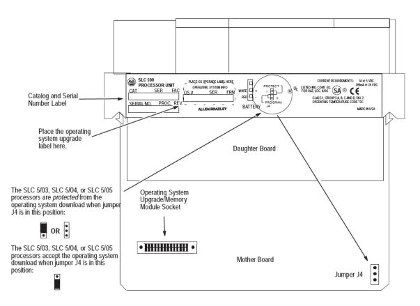
Figure 15 - SLC 500 Processor Component Locations
