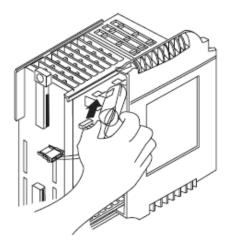
2. Insert the battery connector into the connector port. The connector is keyed to engage with the correct polarity.
