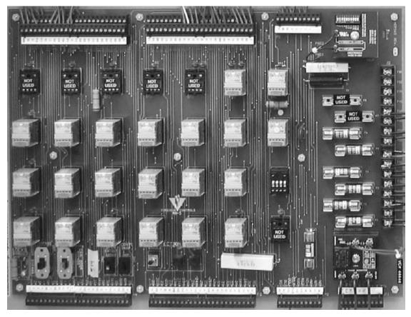
Figure 47 - MH5 Safety Interface Board
