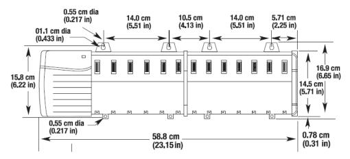
Figure 40 - Allen-Bradley ControlLogix #1756-A13 Chassis (with Power Supply)
