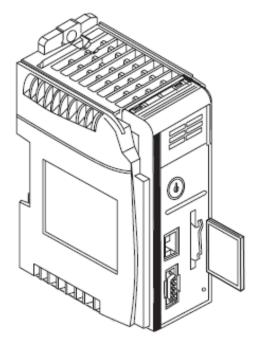
Figure 29 - Allen-Bradley CompactLogix CompactFlash Card Installation
