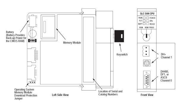
Figure 13 - SLC 5/04 Processors (1747-L541, 1747-L542, or 1747-L543)
