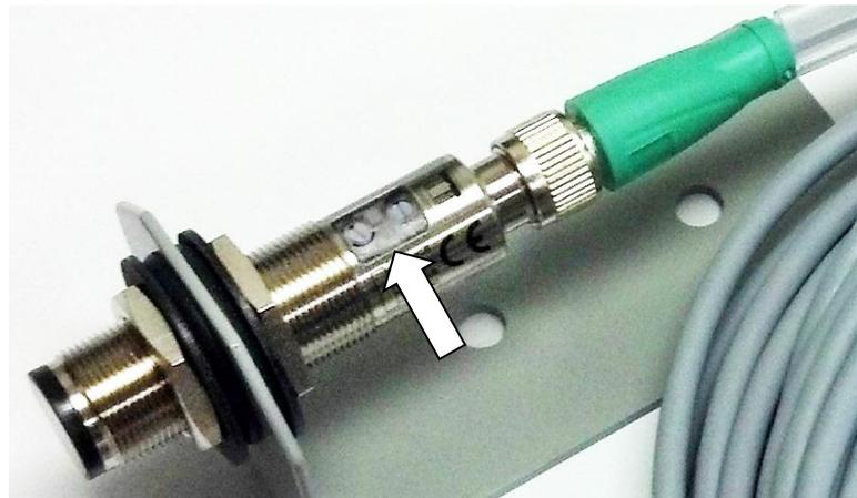
**Figure 78 - Sensor Green POWER LED Indicator**
