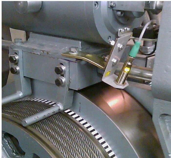
**Figure 8 – Installed ETSD Tape & Sensor**
