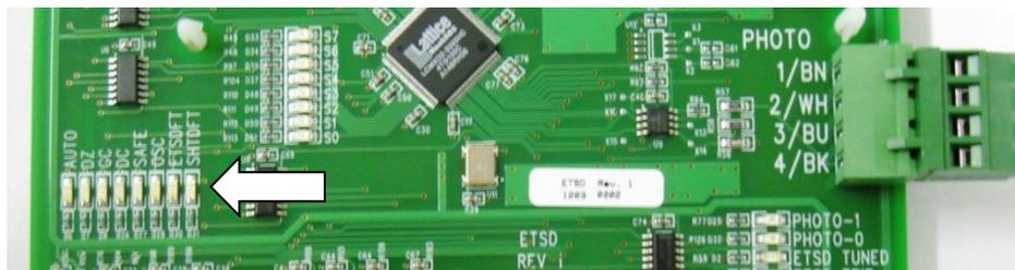
Figure 3 - ETSDFT & SHTDFT Input Indicators
