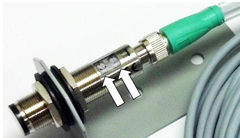
**Figure 13 - L/D Switch (Left) & SENS. Adjustment (Right)**
