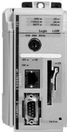
CompactLogix controllers can monitor and control I/O across the 1769 CompactBus, as well as over remote I/O links. CompactLogix controllers can communicate with computers or other processors across RS-232-C (DF1/DH-485 protocol), DeviceNet, ControlNet, and EtherNet/IP networks.
