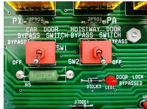
Figure 65 - T1A Board Bypass Switches
