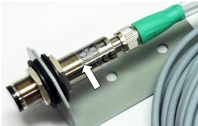
Figure 26: Sensor Green POWER LED Indicator
