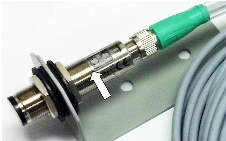
**Figure 52 - Sensor POWER LED Indicator**
