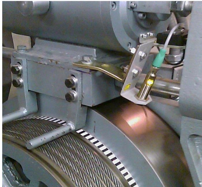
**Figure 23: Installed ETSD Tape & Sensor**
