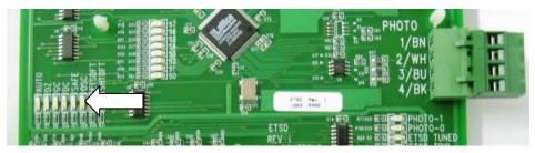
Figure 18: ETSDFT & SHTDFT Input Indicators
